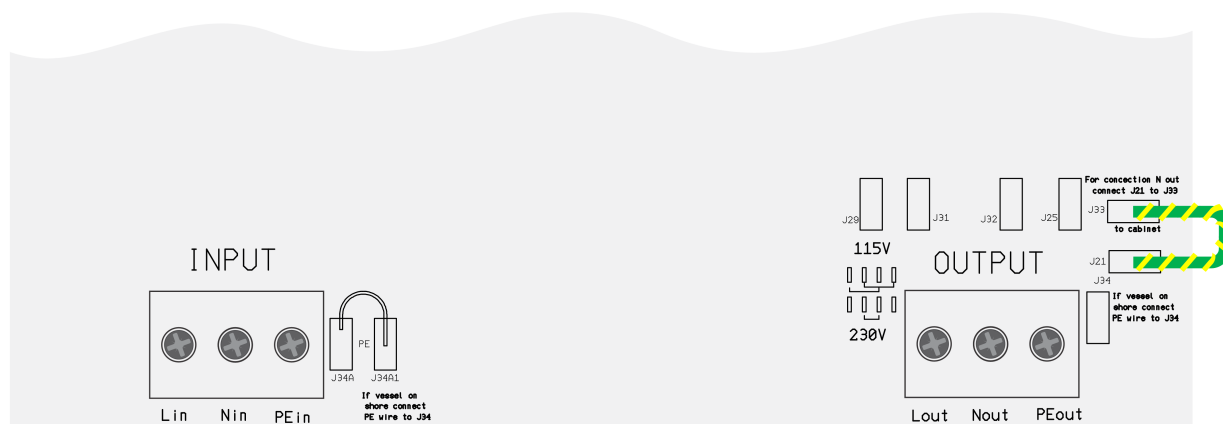
AC output neutral (N) to earth (PE) link.
