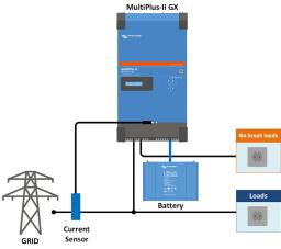
Standard mobile or off-grid application with external current sensor Maximum current sensing range: 50 A resp 100 A
