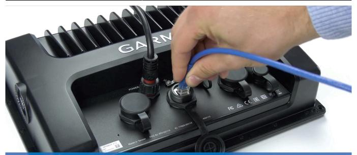
Step 1: Connect UTP into display
