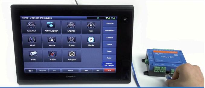
Step 2: connect UTP cable into Victron
