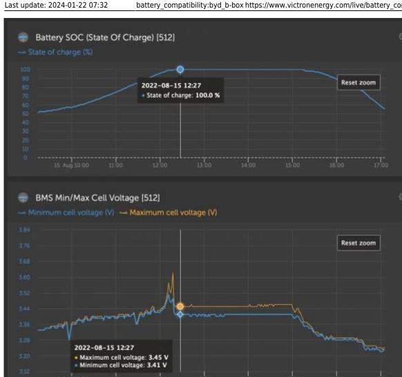
In an imbalanced battery installation, you can see the minimum cell voltage does not rise as much (if at all), compared to the maximum cell voltage. Once the battery is at 100%, the maximum cell voltage does not fall back closely in line with the minimum cell voltage. Any power spikes are disproportionately affecting the high voltage cells, generating alarms, and putting the system at risk of shutting the battery down.
