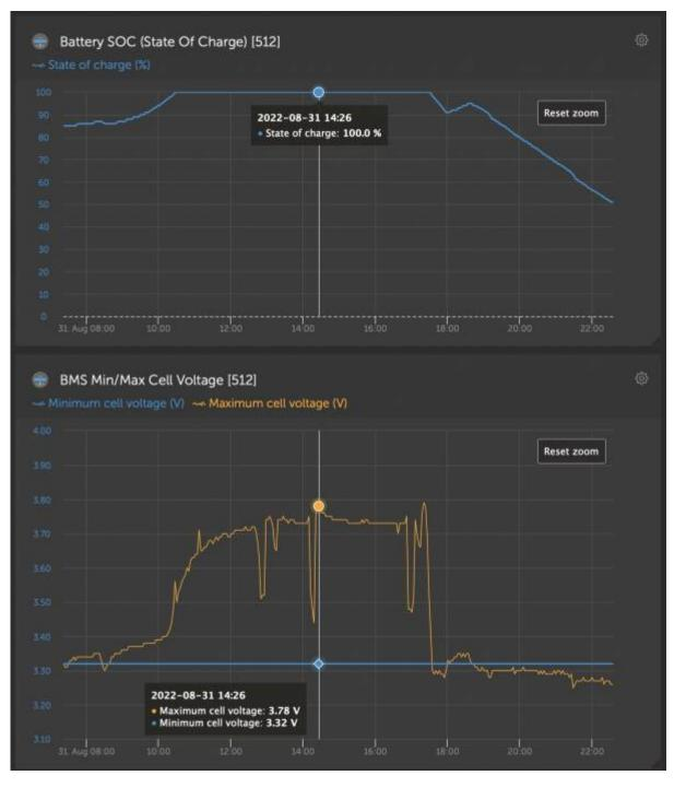
To help the batteries balance quickly, keep the batteries fully charged and the system voltage stable until the errors go away. In an ESS system, set it to 'keep batteries charged', in an off-grid system the fastest way is to either charge / balance the battery before installation, or to fully charge with a generator if not enough solar is available to keep the batteries fully charged.
